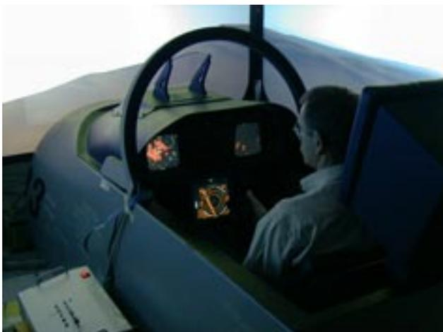
From the foregoing analyses, CMC catalogued a number of display integration, interpretation and mission impact concerns, used to later formulate the design objectives for the development of new rapid prototype displays elements for the CF-18. In order to implement the display element design objectives, the CMC HFE Team made modifications to the HFE test and evaluation apparatus to support a simulated CF-18 operational environment. These included the
