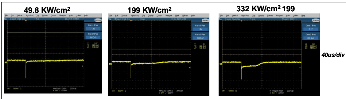
Figure 6: Recovery time for APD only at different power levels
